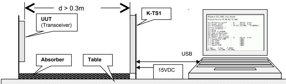
Fig. 11: Typical arrangement of a test-stand
