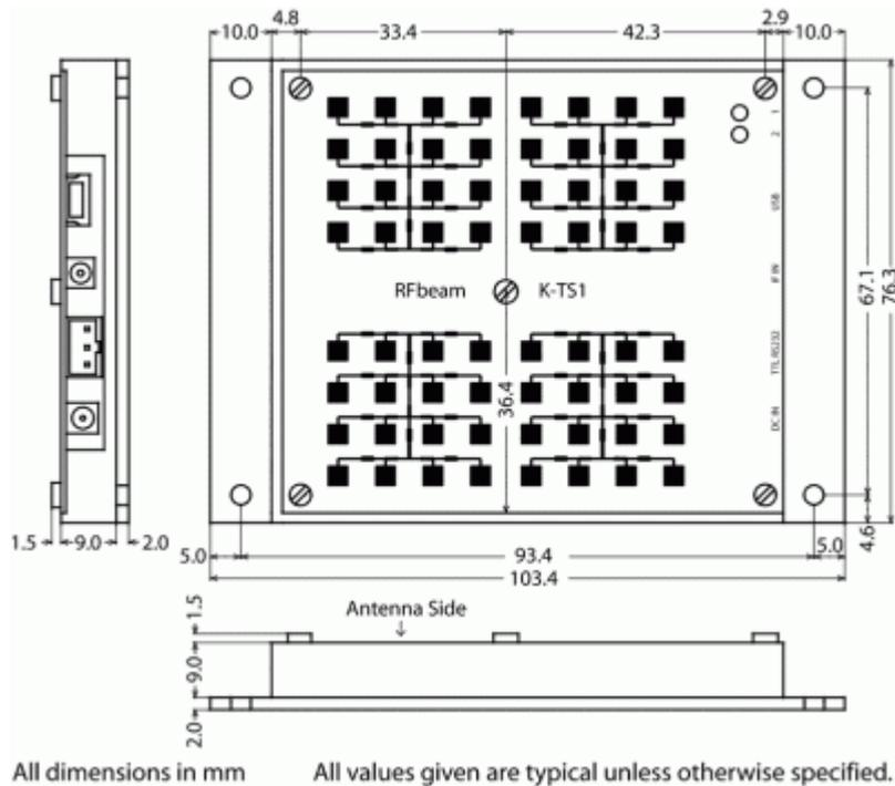
Fig. 13: Mechanical dimensions
