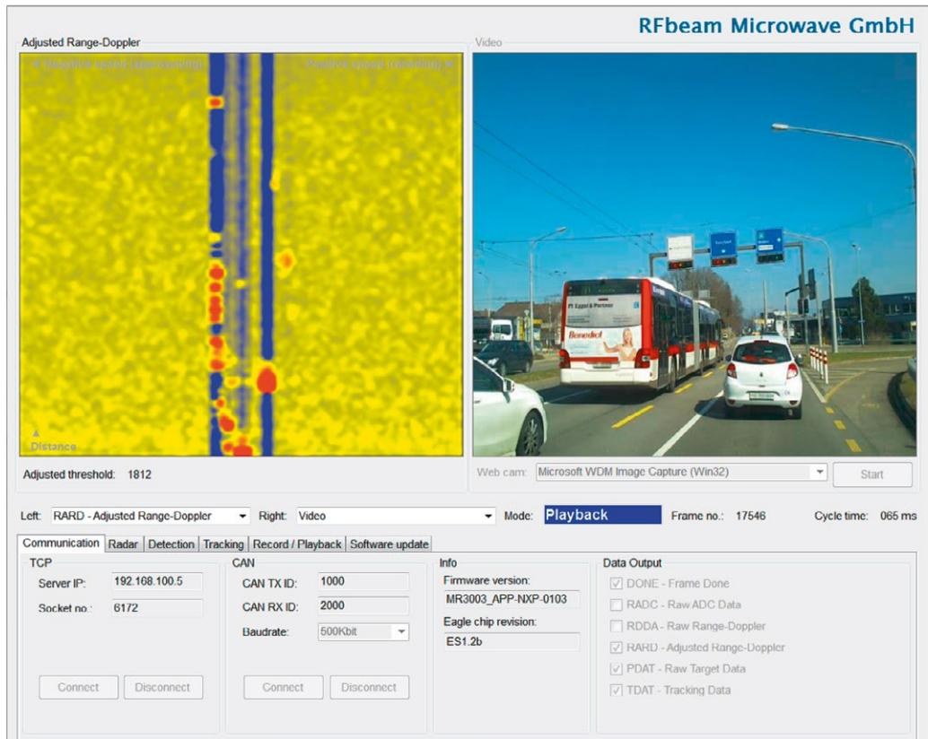
Figure 1: Control panel GUI overview
