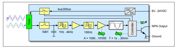
Fig. 4: Block Diagram
