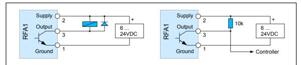
Fig. 5: Examples: Left Relais, Right Controller
