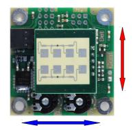
RFA1 can be mounted as shown on the left to get horizontally a "narrow field". Rotating the module by 90° results in a wider field.
