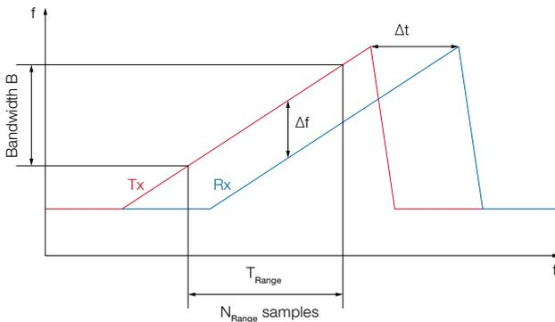
To measure the speed the V-MD3 sends  $N_{\text{Speed}}$  FMCW range chirps spaced with the time  $T_{\text{Speed}}$ . These multiple chirps are called a frame. Each reflected chirp is processed by means of a FFT to detect the range of the objects as described in the last chapter (range-FFT). The range-FFT corresponding to each chirp will have magnitude peaks in the same location, but with a different phase. The measured phase difference between the chirps corresponds
