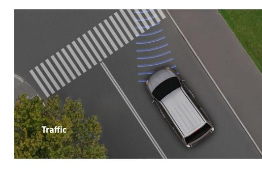
RFbeam offers a wide range of sensors for use in traffic applications. Radar is known for its speed measurement capabilities. In addition, Radar can also measure direction, distance and angle of dynamic and static objects in all weather conditions. This makes radar the number 1 choice for many traffic applications.
